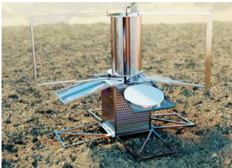
Figure 1: Notional wind powered version of the Long-Life In-situ Solar System Explorer Venus Probe Concept
