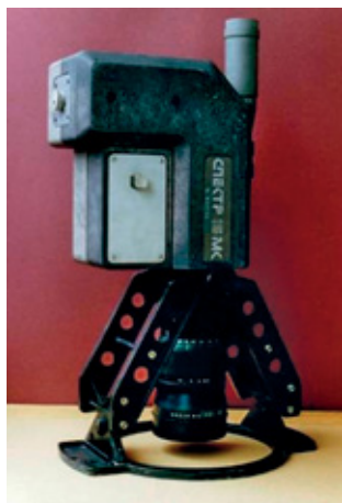
Fig. 6. Trace spectrometer Spectrum 15 developed for the flight of G. Ivanov and N. Rukavishnikov on Salyut 6
