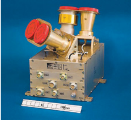
One of the two instruments within Plasma-F suite: Energetic Particles Monitor (MEP)
