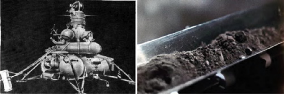
Luna 16 autonomous sample collection from a basaltic terrain in eastern Mare Fecunditatis: the Luna 16 lander (left); image of the bulk sample (soil and pebbles) returned to Earth for analyses (right)
