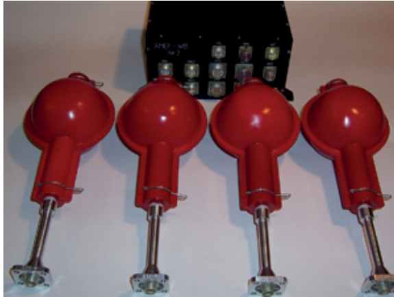
Fig. 27. Instrument AMEF-WB for measurement electric and magnetic fields in the frequency range 0–1 MHz of the Resonance project
