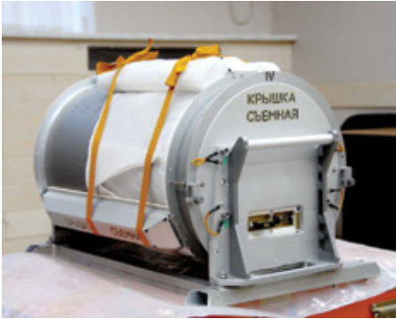
Chibis-M microsatellite in the transportation/launch container to be installed in Progress-M cargo ship
