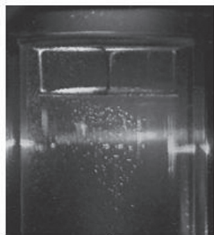
fig. 10. Typical image of a stationary 3D structure (cloud) in the vicinity near the net-shaped electrode
