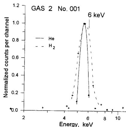
Fig. 2 Energy spectra of originally 6 keV  $H_2$  molecules and He atoms after the foil of No. 001 GAS 2 instrument.
