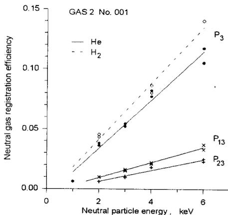
Fig. 7 The energy dependence of the  $P_3$ ,  $P_{13}$ ,  $P_{23}$  absolute efficiencies of No. 001 GAS 2 instruments for helium atoms and hydrogen molecules.
