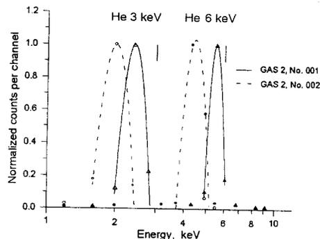
Fig. 3 Energy spectra of originally 3 keV and 6 keV He atoms after the foils of No. 001 and No. 002 GAS 2 instruments.
