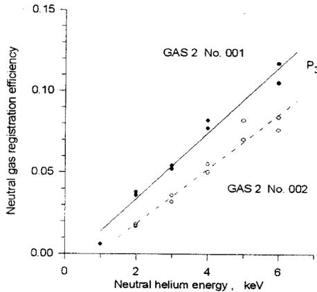
Fig. 6 The energy dependence of the absolute efficiencies of  $D_3$  detectors of No. 001 and No.002 GAS 2 instruments for helium atoms.
