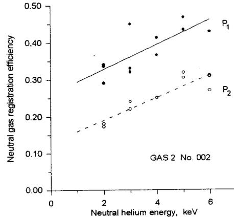
Fig. 5 The energy dependence of the absolute efficiency of  $D_{1,2}$  detectors of No. 002 GAS 2 instruments for helium atoms.
