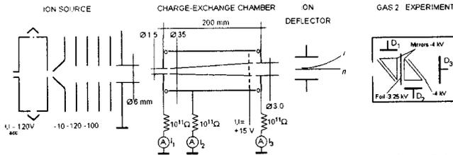
Fig. 4 Scheme of MPAE facility used for the absolute calibration of the GAS 2 instrument.
