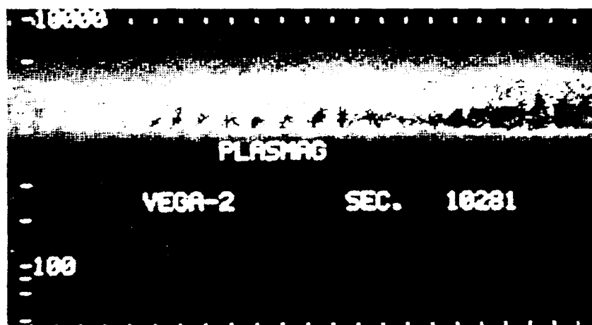
Fig. 4. Colour-coded representation of the intensities (see colour-table in Fig. 3) vs. energy/charge (vertical axis) and time (horizontal axis with 10 s time-marks) of cometary ions measured by the VEGA-2 CRA within the 'cometary plasma region' from 7:00 to 7:04 UT. Notice the quasi-periodical occurrence of cometary ions in lumps.
