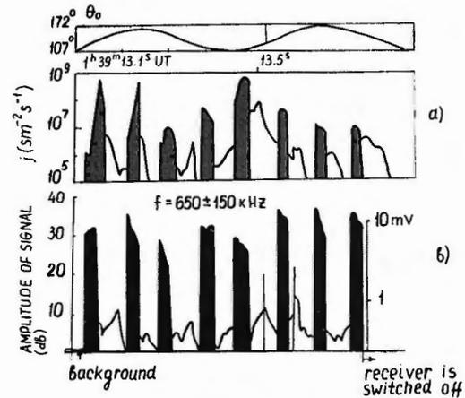
Figure 3: Bursts of electrons ( $E > 8$  keV) observed at the rocket between electron pulses injected downwards (launch of February 15, 1975) and bursts of radiation in the whistler range simultaneously received at separated nose cone.
