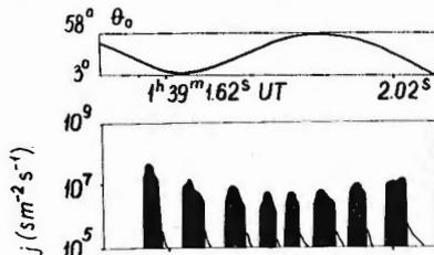
Figure 2: Fluxes of electrons ( $E > 8$  keV) measured aboard the rocket during upward injected pulses (launch of February 15, 1975).
