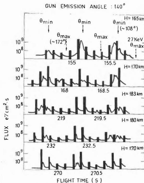
Figure 1: Fluxes of electrons ( $E > 8$  keV) measured aboard the rocket during several series of electron pulses injected downwards (launch of February 15, 1975) and bursts of precipitated electrons in pauses between injected pulses.
