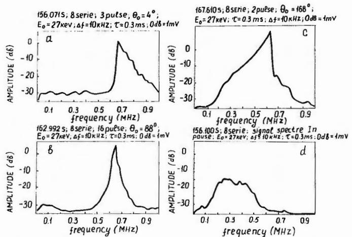
Figure 4: Frequency spectra of signals received in the whistler range at the nose cone during downwards injection of electron pulses with different injection angles (a, b and c) and in the pause between injected downwards pulses (d).
